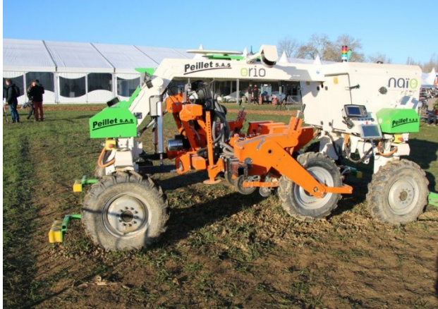
Naïo Orio is equipped with a Stanhay precision seeder.
